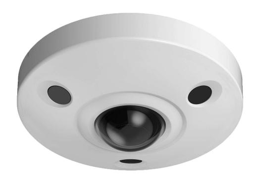
1/1.7" 12Megapixel progressive scan STARVIS CMOS • H.265/H.264 triple-stream encoding • Max 25fps@12M(4000x3000) • Multiple dewarped Mode • Day/Night(ICR), 3DNR, AWB, AGC, BLC • Smart detection • Intelligent Function • Max. IR LEDs length 10m • Micro SD memory, IP67, IK10, PoE
