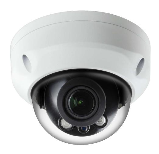
1/2.5" 8 Megapixel progressive scan STARVIS CMOS • H.265 & H.264 dual-stream encoding • 15fps@4K(3840x2160), 25/30fps@3M(2304x1296) • Day/Night(ICR), 3DNR, AWB, AGC, BLC • Multiple network monitoring: Web viewer, CMS(DSS/PSS) & DMSS • 2.7~12mm motorized lens • Max. IR LEDs Length 50m • Micro SD card slot • IP67, IK10 • PoE
