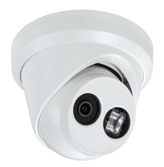
1/2.5" (8 MP) Progressive Scan CMOS • Up to 3840 x 2160 Resolution @ 15 fps • 2.8 / 4mm Fixed Lens • EXIR 2.0 Range Up to 100 ft (30 m) • H.265+/H.265/H.264+/H.264 • 120dB True WDR • IP67 Protection • Durable Metal Housing • 12 VDC 25% (PoE 802.3af), maximum 7.5 W
