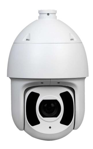
1/2.8" 2 Megapixel STARVIS™ CMOS • Powerful 45x Optical Zoom • Starlight technology • Max. 50/60fps@1080P • Auto-tracking and IVS • IR distance up to 820ft • Support PoE+ • IP67, IK10
