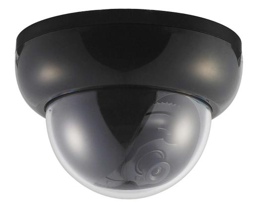
1/2.9 inch SONY CMOS (IMX-222 • IMX-322) • HD-SDI (1080P • 720P • 720P CROP) • Extended Serial Digital Interface • 1 Lux at F1.2 • 0.1 Lux (B/W) • OSD Controlled • DNR (Digital Noise Reduction) • Smart IR • WDR (Wide Dynamic Range) Day & Night (ICR Option) • D.ZOOM • Privacy • Image Conversion • Easy Installation Fixed Lens 2.9mm • 3.6mm • 3.7mm • 4mm • 4.3mm • 6mm
