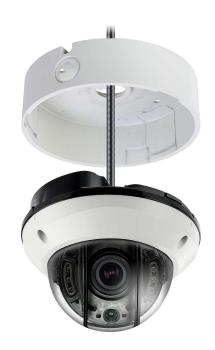
1/1.7 inch SONY CMOS (IMX-226) • 0 Lux at IR On (IR LED 10 pcs) / Upgraded Waterproof Housing (IP 68 rating) • DNR (Digital Noise Reduction) / WDR (Wide Dynamic Range) • Day & Night (ICR Option) / Easy Installation • ICR V/F lens, DC Auto IRIS V/F Lens, DC Auto IRIS & TDN V/F Lens • Focal Length : 3.6~10mm
