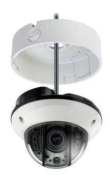
1/2.9 inch SONY CMOS (IMX-326) / Upgraded Waterproof Housing (IP 68 rating) • High Definition Serial Digital Interface / 0 Lux at IR On (IR04) • Digital WDR (Wide Dynamic Range) / DNR (Digital Noise Reduction) / Day & Night (ICR Option) • ICR V/F lens, DC Auto IRIS V/F Lens, DC Auto IRIS & TDN V/F Lens • Focal Length : 2.8~12mm
